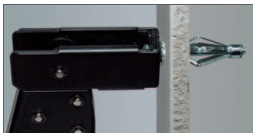
3. Hang the screw head by the special tool (HQ series), then use the tool-gun until the complete opening of the anchor as showed in the picture.
